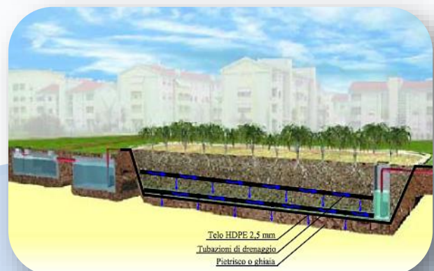
Detail of the preliminary project, on site soil treatment tanks
